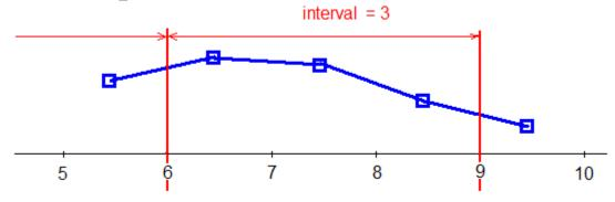
Now, all the data of the new calculated interval between t = 6s and t = 9s can be retrieved using interpolation.
