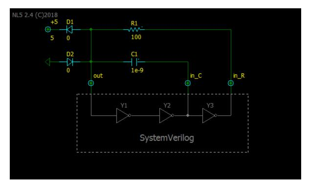
Digital part (Y1, Y2, Y3) of the circuit is disabled, since it will be simulated by SystemVerilog. Labels "out", "in\_C", and "in\_R" are used for passing signals between analog and digital parts.
