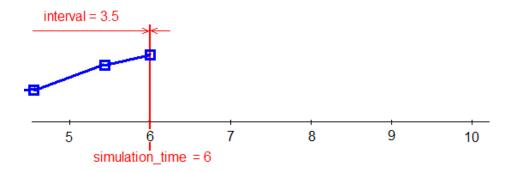
When NL5 SimulateInterval is called again with requested interval = 3.5s, simulation step is restored back to 1s, and simulation continues:
