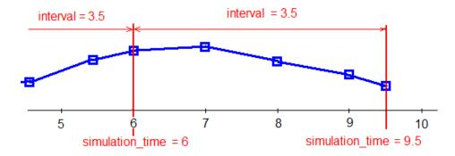
In this call, simulation step was also decreased at the end of the interval from 1s down to 0.5s, in order to stop exactly at 9.5s.
