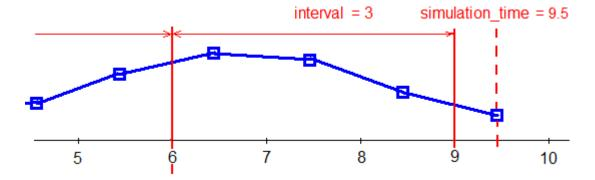
Using NL5 Simulate function provides the best simulation performance. It won't decrease simulation step at the end of current linear range, so that there is no need to restore the step back as simulation continues. Thus, the simulation will be performed in a fastest manner, regardless of simulation interruptions.
